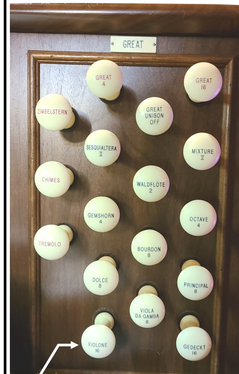
This controls the biggest pipes in the façade. This is also borrowed by the Pedal division. (Go to Pg. 24)
